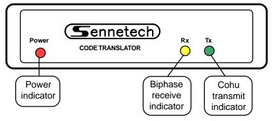
The code translator works in simplex mode without using the receiver response, so only one pair of data wires is required. The response lines can be connected to other equipment for processing status and alarm data.
