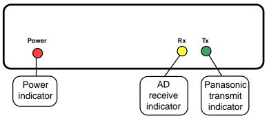
The Rx indicator will flash when manchester code is being received. Since AD manchester code is repeating, it will flicker continuously while a camera is being moved. Panasonic code is repeated at a slower rate.
