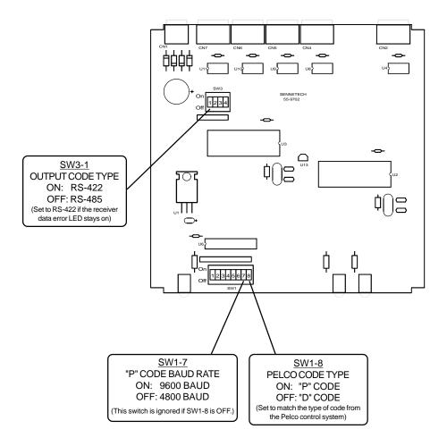
If the code translator is configured to receive "D" code, the baud rate is automatically set to 2400. For "P" code, the available baud rates are 4800 and 9600.
