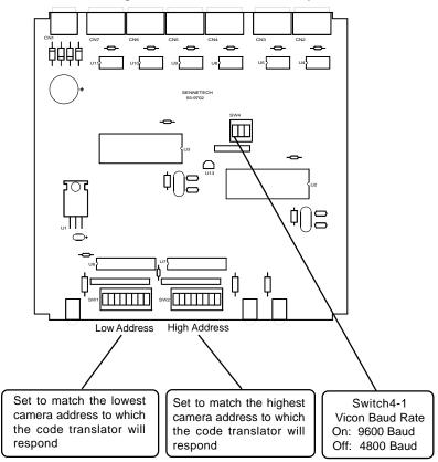
The code translator will appear as a group of cameras to the controller. To prevent interference between the responses from the code translator and any Vicon cameras in the system, set the switches to exclude any Vicon camera addresses.
