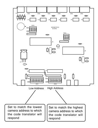
The code translator will appear as a group of cameras to the controller. To prevent interference between the responses from the code translator and any Vicon cameras in the system, set the switches to include only the Javelin camera addresses.
