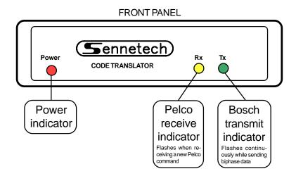
The Rx indicator will flash whenever there is data from the Pelco controller. If the input lines have reversed polarity, the Rx indicator will be on solidly. Biphase code is repeating so the Tx indicator will continue to flash while the camera is moving.
