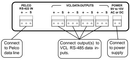
The Rx LED will light when there is any data on the input lines.
