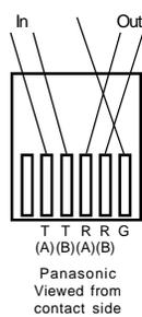
Removable edge connector. Insert a small screwdriver in the upper slot to force open the wire clamp. Push all the way in to open fully. Place stripped wire end(s) in the open clamp and withdraw screwdriver.
