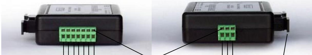
Connect power to the PWR inputs. Do not connect power wires to the Gnd.
